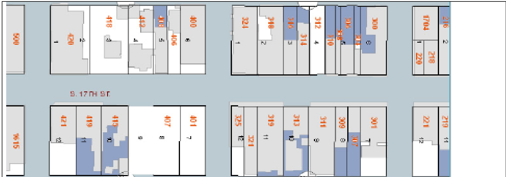
This diagram illustrates the maintenance of appropriate setbacks in a commercial district. The areas highlighted in blue show the appropriate location for additions and parking.
